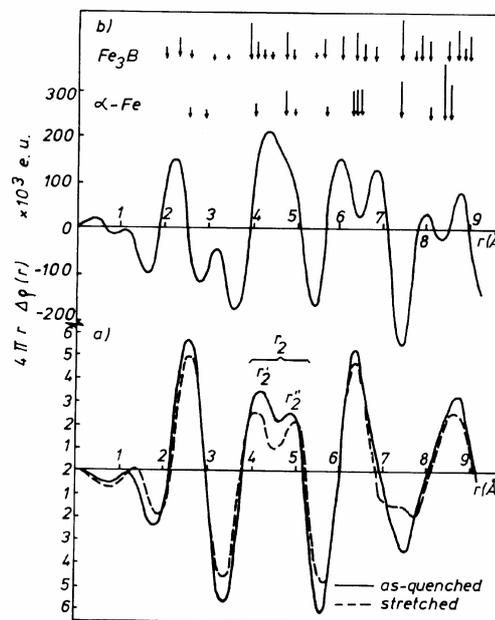
Fig. 9. The radial distribution functions for the  $\text{Fe}_{80}\text{B}_{20}$  glassy ribbon. (a) Reduced RDF before and after deformation. (b) Differential RDF: (as-quenched state)– (stretched state).
