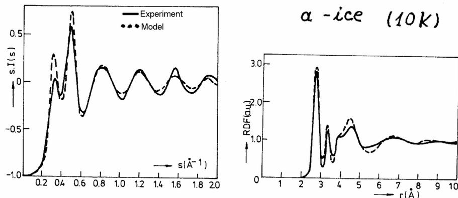
Fig. 2. The structure factor and the reduced (differential) radial distribution function of amorphous ice deposited and studied at 10 K (---) compared with those calculated from a structural model with 156 atoms (—). The model contains only even rings of atoms (6 and 8-fold rings) [8].
