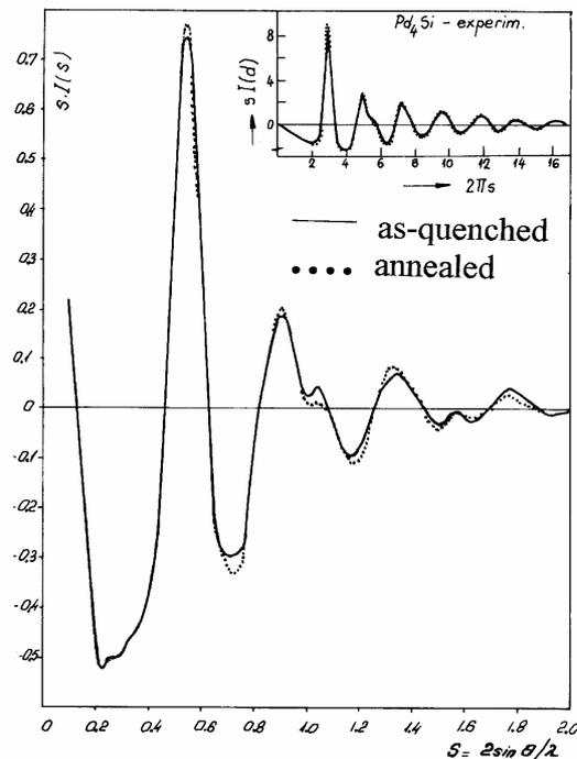
Fig. 10. The reduced radial distribution function for glassy  $\text{Pd}_4\text{Si}$ . The experimental results and the curve calculated from the DRPSU model. — initial relaxed configuration; --- final relaxed configuration (annealed) experimental: — as-quenched --- annealed, 250 °C, 40 min.
