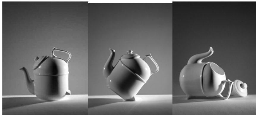
Figure 0.3 The Ronnefeldt “tilting” teapot. Put leaves on the internal shelf (not visible, but just above and parallel to the ridge that can be seen running around the body of the teapot), fill with hot water, and lay the teapot on its back. As the tea darkens, tilt the pot. Finally, when the tea is done, stand the teapot vertically, so the water no longer touches the leaves and the brew does not become bitter. 4
