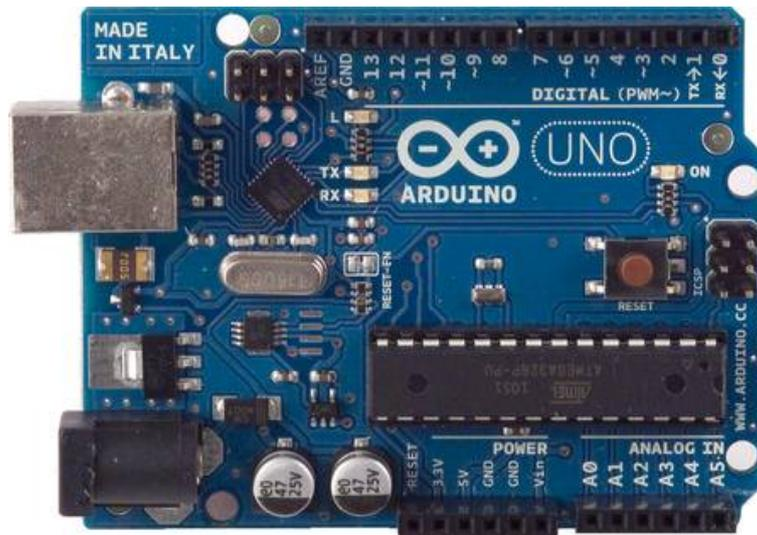
**Figure No 05. Arduino Uno Rev3-Main Board**
