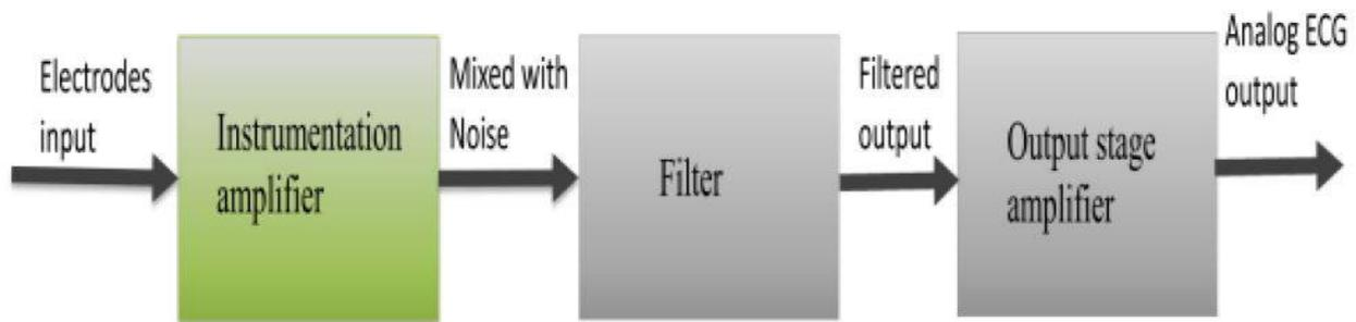
**Figure No 3: Block diagram of ECG Sensor**
