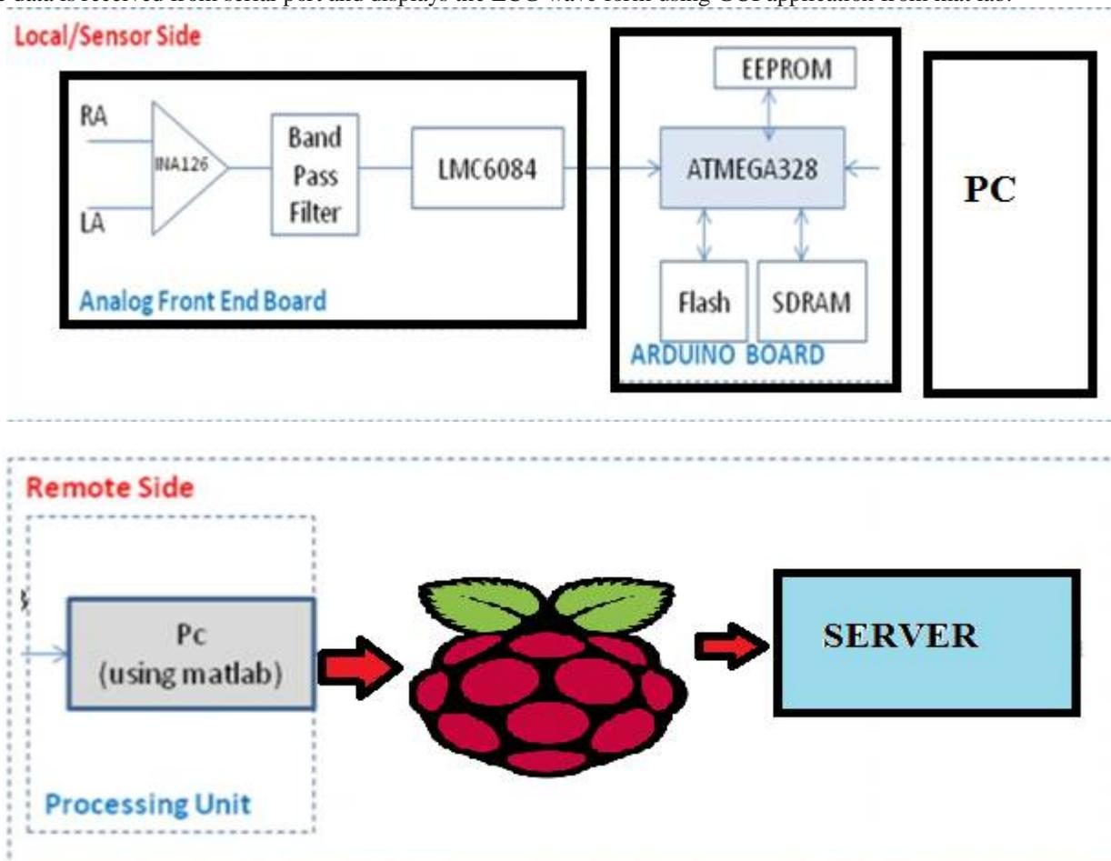
Figure No 02. Block diagram of the circuit
