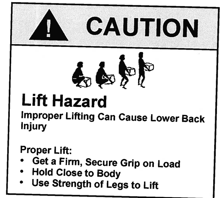
FIGURE 53.7. Example of a proposed sign warning against a lift hazard.
