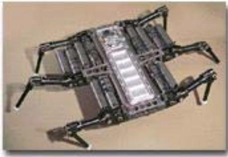
←----- Robot worker capable of carrying payload on its back and using all six tentacles as arms or crawlers
