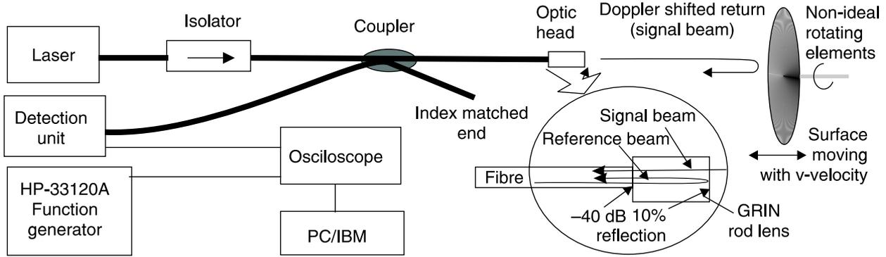
Fig. 1. Schematic view of the SRFP fibre interferometer.
