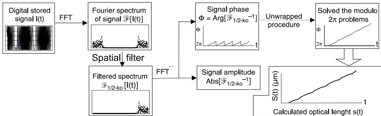
Fig. 2. Diagram of applied DFFT method.
