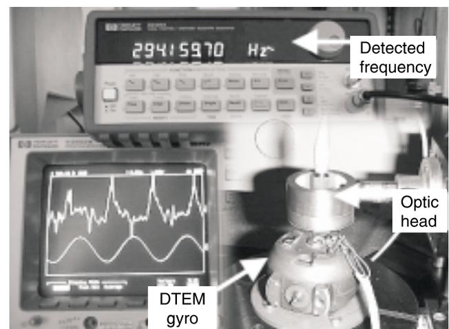
Fig. 8. View of SRFP system with measured DTEM gyro (detected rotation speed  $17650 \text{ turns/min}$ ).
