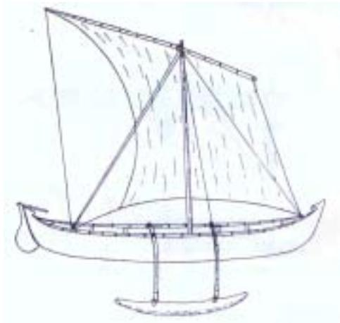
**Fig 6- A Kilakarai outrigger fishing-boat, with two booms**
