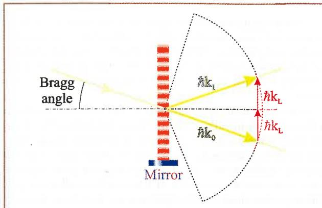
▲ **Fig. 2:** Diffraction of a matter wave in the Bragg regime: one photon is absorbed in one of the two traveling waves forming the standing wave and is emitted by a stimulated process in the other traveling wave. During this process, the kinetic energy of the particle (hence the modulus of the atomic wavevector) and the total momentum are both conserved.
