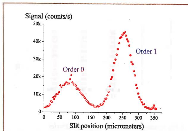
▲ **Fig. 3:** Bragg diffraction of a lithium atomic wave by light. The intensity in the diffraction orders 0 and 1 is recorded by moving the detector. The laser standing wave has been adjusted to give a high diffraction probability into the first order. In a separate experiment, we have verified the absence of other diffraction orders, in agreement with the theory of Bragg diffraction
