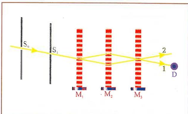
▲ **Fig. 1:** Scheme of a three grating Mach-Zehnder interferometer. After collimation by the slits  $S_0$  and  $S_1$ , the matter wave travels through the diffraction gratings which are either material gratings or laser standing waves created by reflection of traveling waves on the mirrors  $M_1$ ,  $M_2$  and  $M_3$ . A detector  $D$  is placed on one of the two outputs of the interferometer, labeled 1 and 2 in the figure. The interference signals on both outputs have opposite phases.
