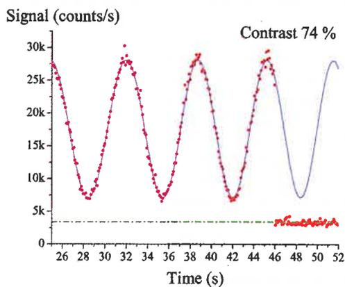
▲ **Fig. 4:** Atomic interference fringes recorded by moving the position of the third grating of the interferometer. Each point corresponds to a counting time of 0.1 s. Once the background signal (recorded on the right of the figure) has been removed, the measured fringe contrast is 74%.
