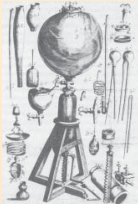
Air pump built by Robert Boyle and Robert Hooke for creating a vacuum (Bancroft Library, University of California, Berkeley)
