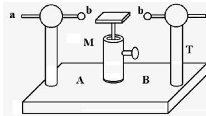
**Figure 3** The apparatus described by Izarn in 1804. Author's reconstruction of IZARN (1804), fig. 53, plate III, facing p. 130.
